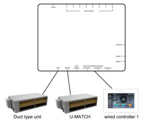
Fig 5.2 Communication wire connection
