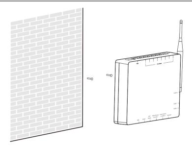
Fig 5.4 Vertical installation diagram
