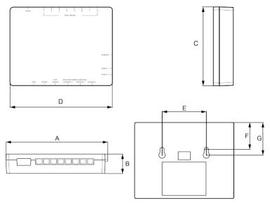
Fig 5.1 Zone control interface size (unit: mm)
